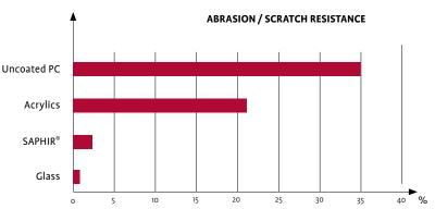
The abrasion test shows the decrease in transparency after abrasion. SAPHIR® has glass-like properties thanks to the protecting hard coat.
