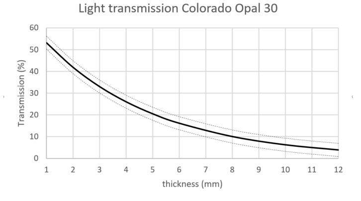
This graph is also valid for the Colorado UV version. These are typical light transmissions. Product specification allows for a tolerance on these values.
